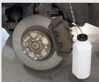
Waste Fluid Bottle connects to vehicle's bleeder screws and chain with hook holds bottle in place.
